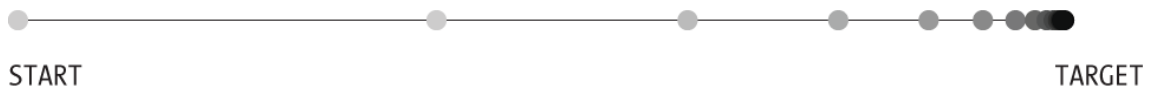
Figure 5-1. Easing changes the number of steps it takes to move from one place to another
